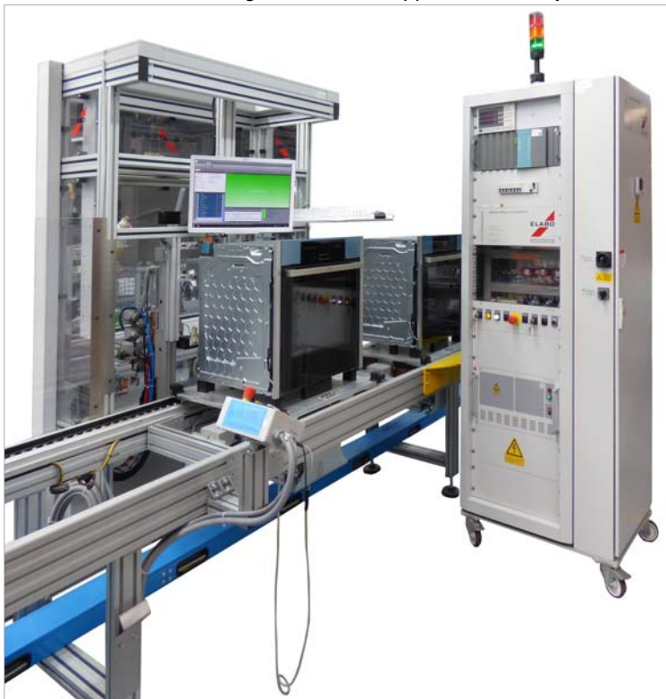
Photo 1: End-of-line testing of household appliances with systems from ELABO
